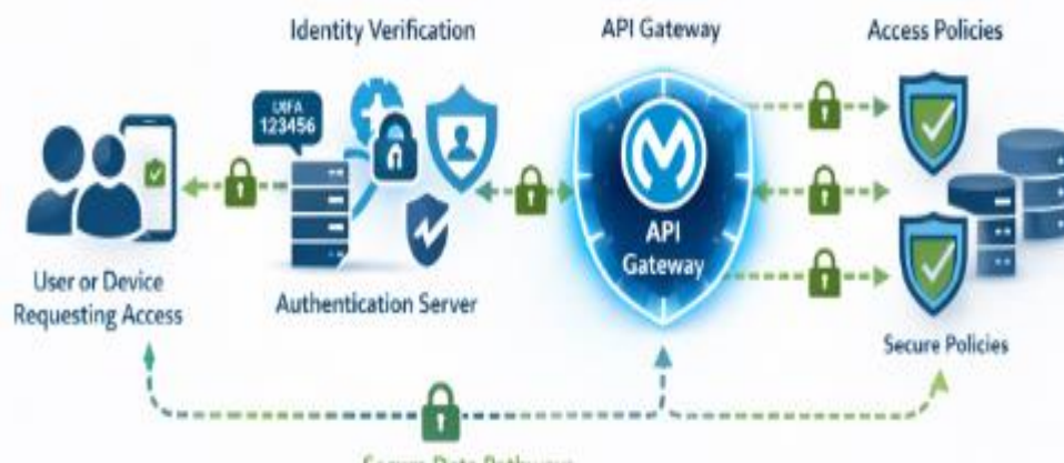
Figure 2: Zero-Trust Security Model for API Access
