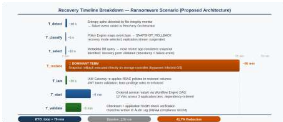
Fig. 2. Recovery timeline breakdown for ransomware scenario showing per-step latency contributions. T_restore dominates at ~55 minutes; total RTO = ~70 minutes (41.7% reduction vs. 120-minute baseline).
